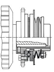
Combined with a flexible coupling, the OPTI torque connects drive and driven shafts, accomodating angular, axial and radial shaft misalignments, while also providing overload protection.
