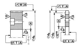
Extended hub (page 5): For wider drive elements, the drive element is bolted to the output flange. Support of the drive element is either by a customer provided bearing or bushing, or one that is integral to the OPTI torque, as in the models 460.\_\_\_.2 and 460.\_\_\_.5.
