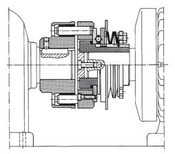
The extented hub and integral bushing of the OPTI torque makes it ideally suited for wider drive elements, such as this pulley. With the OPTI torque installed with the pulley inward, overhung load on the drive shaft is minimized, and easy access is provided for torque adjustments.
