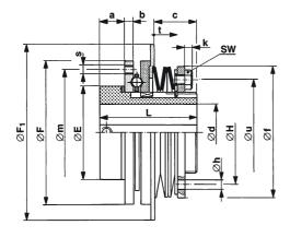
Type 460.\_1\_.1 OPTI torque with extended hub
