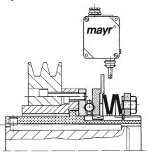
Preferably OPTI torque should be held on the shaft by means of a clamp plate, as shown in the figure below.
