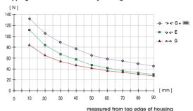
Order no.: GZ25-35 GZ25-35 Е Drive: pneum. Stroke per jaw [mm]: 5 5 Stroke per jaw [°]: Gripping torque in closing [Nm]: 5,4 Gripping torque in opening [Nm]: Self-locking via: Spring Spring Closing time/opening time [s]: 0,2/0,3 0,2/0,2 Repeatability ± [mm]: 0,1 Min./max. operating pressure [bar]: Air volume per cycle [cm³]: 6 Min./max. operating temperature [°C]: Temp. resistant version up to 150° C [add to part number]: Weight [kg]: 0,253 0,313
