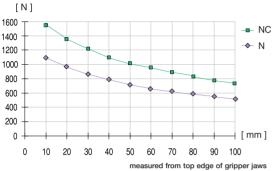
Order no.: **GG70** NC N Drive: Stroke per jaw [°]: 35 35 Gripping torque in closing and opening [Nm]: Gripping torque in closing [Nm]: 122 Self-locking via: Closing time/opening time [s]: 0.3 Repeatability ± [mm]: 0,05 Min./max. operating pressure [bar]: 3/10 5/10 Air volume per cycle [cm³]: Min./max. operating temperature. [°C]: Temp. resistant version up to 150°C [add to part number]: Piston diameter [mm]: Weight [kg]: 6,8 5,9
