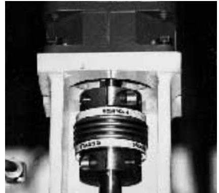
Series AKN Application – servo-drive / milling machine
