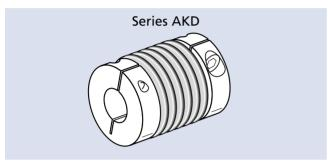
To connect two shafts, backlash free shaft-hub connection using collet clamps. For torques between 18 – 500 Nm.
