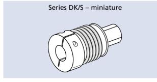
To connect two shafts, backlashfree shaft-hub connection using a collet clamp and an expanding clamp. For torques between 0.40 – 10 Nm.
