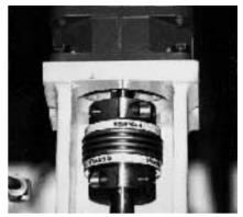
**Series AKN**Application – servo-drive / milling machine
