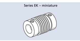
To connect two shafts, backlashfree shaft-hub connection using set screws. For torques between 0.10 – 10 Nm.
