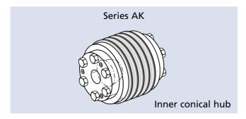
To connect two shafts, backlashfree shaft-hub connection using conical hubs. For torques between 30 – 5000 Nm.
