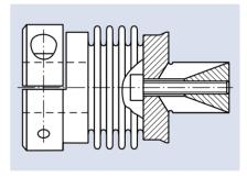
**Series AKN/S**Model with collet and expanding clamps
