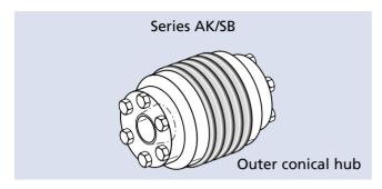
To connect two shafts, backlash free shaft-hub connection using outer conical hubs, contracting disc, no releasing screw required, release during dismantling. For torques between 18 – 5000 Nm.
